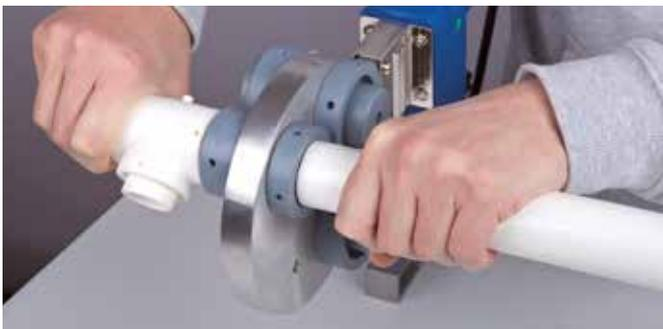
Fig. 12: Heating up fitting profile and pipe end.
