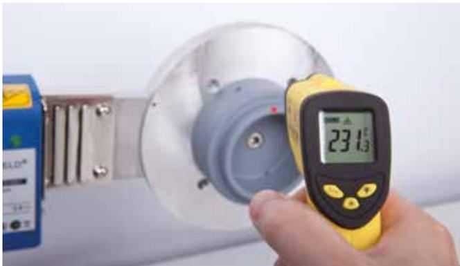
Fig. 4: Example of a surface temperature measurement on a front bead of a heating element  $\varnothing$  75 mm
