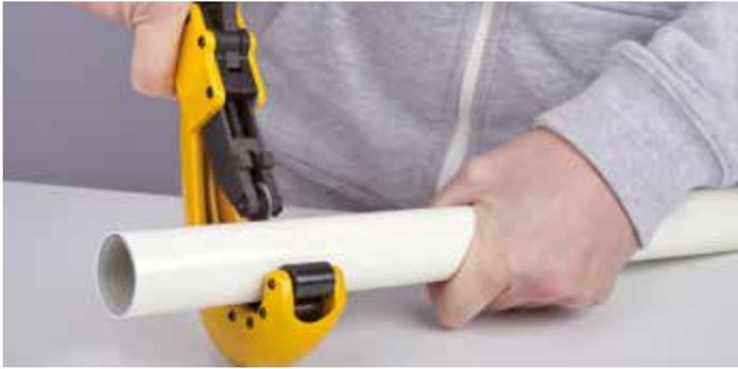
Fig. 6: Cut the multilayer pipe of the WRW welding system (diameter range  $\varnothing$  20 mm to  $\varnothing$  75 mm) right angled with a pipe cutter.
