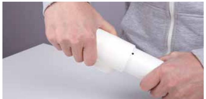
Fig. 13: Join pipe and fitting up to the marking.
